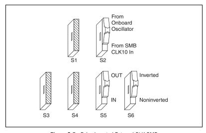
Figure C-5. Drive Inverted External CLK SMB
